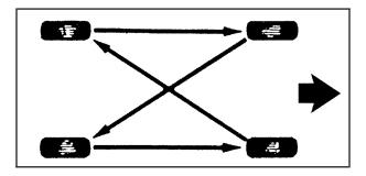
When rotating P235/50R17 size tires or 255/45ZR18 size tires, always use the correct rotation pattern shown here.
